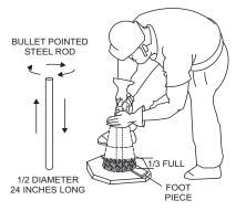
Figure 35-A. Slump Test (1/3 Full)
